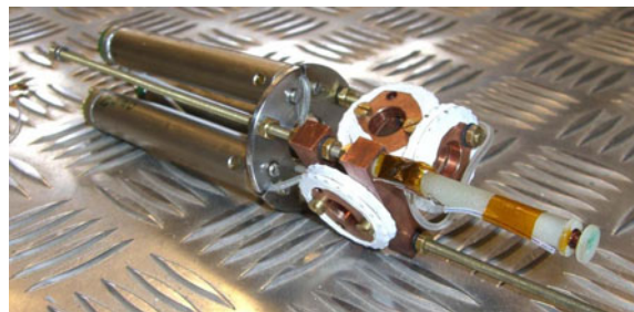
Figure 2. The 3-axis SQUID magnetometry system used for these measurements.
