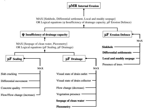
Figure 5: Internal Erosion assessment – Case of dams with concrete facing (direct indicators are indicated by bold type)
