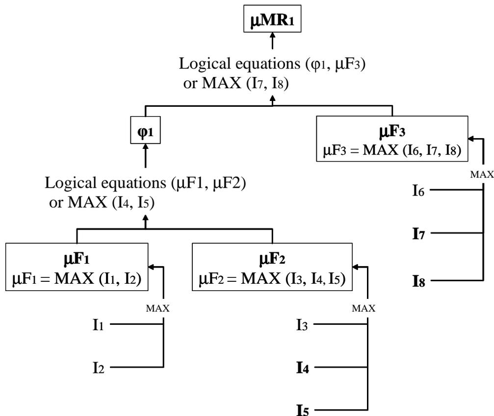
**Figure 3: Performance assessment modelling – direct indicators are indicated by bold type –  $I_j$  = indicator  $j$  -  $\mu F_i$  = Performance of Function  $i$  -  $\mu MR1$  = Performance related to the failure mode MR1 -  $\phi 1$  = phenomenon 1**
