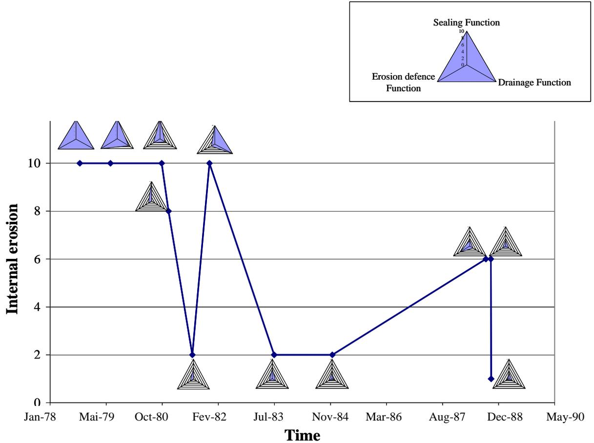
**Figure 6: Assessment of the performance through time for the Sapins Dam – The line represents the assessment of the performance related to internal erosion – A radar diagram showing the performance of the sealing function, the drainage function and the erosion defence function is associated to each assessment time**
