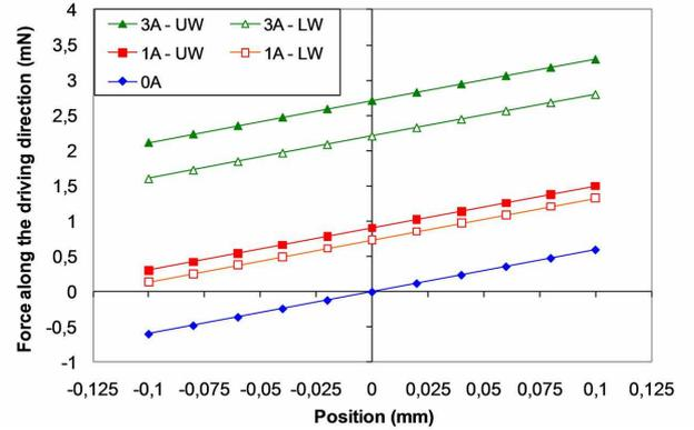
Fig. 4. Evolution of the force along the displacement direction in function of the MPM position between two discrete positions for different driving current values (0 A, 1 A and 3 A) with using the UW and LW
