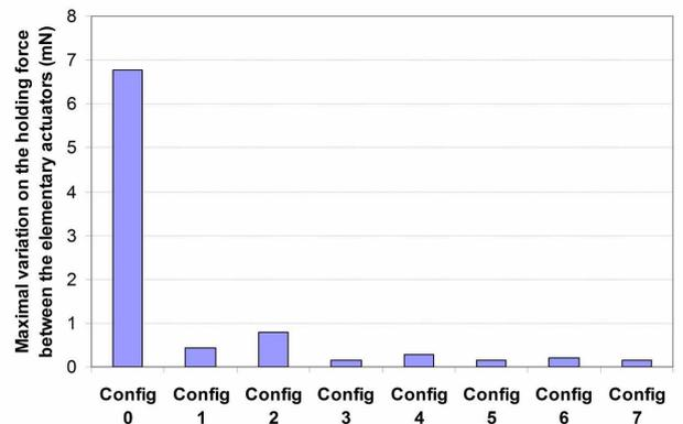
Fig. 7. Evolution of the maximal holding force variation between the elementary actuators in function of the configurations studied
