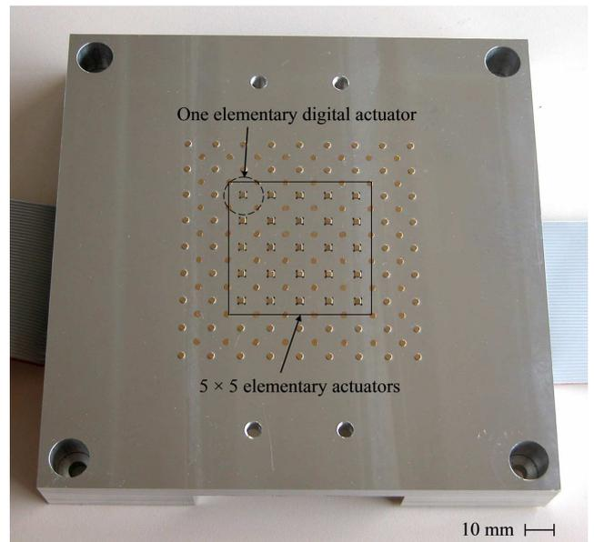
Fig. 9. Overall view of the experimental prototype
