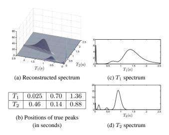
Fig. 4. Reconstruction of 2D NMR experimental data
