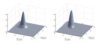
Fig. 3. Reconstruction of a 2D NMR spectrum using the proposed algorithm (left) and the approach of [3] (right). In both cases, the normalized mean square error is about 17%
