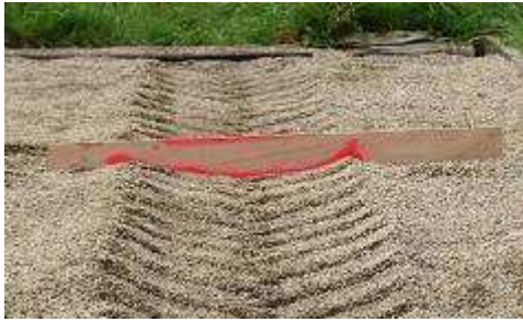
Photo 7: Tracing of rut profile
