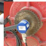
(c) – inductive sensor for spreader speed measure
