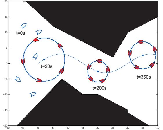
Fig. 2. Simulation of five agents governed by the control law (6) where  $\mathbf{G}(t) = \mathbf{S}_{R(t)} \mathbf{T}_{c(t)}$ . The circular formation with time-varying radius tracks the time-varying center reference in order to avoid the obstacles (black blocks).
