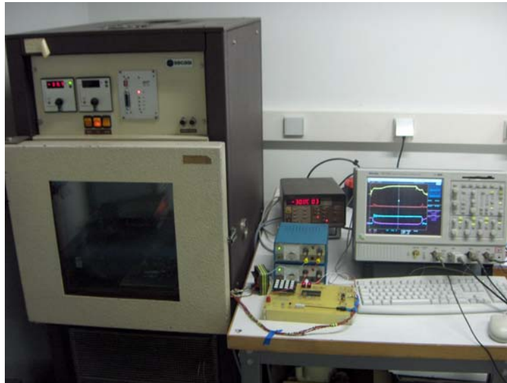
Figure 17 – Overview of the complete switching test bench
