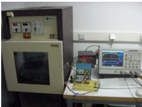
Fig.5 – Hard-switching test bench at low temperature
