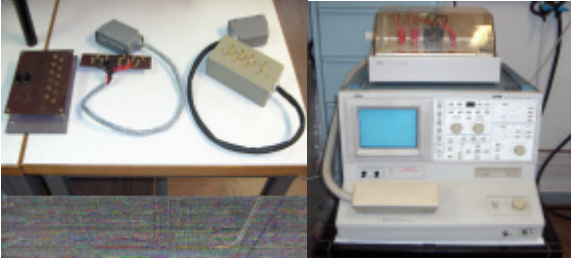
Fig.2 – Specific cable design for TEKTRONIX 371A for low and high temperature operations
