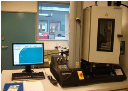
Figure 11 – Climatic chamber allowing ambient temperature from 175K up to 575K
