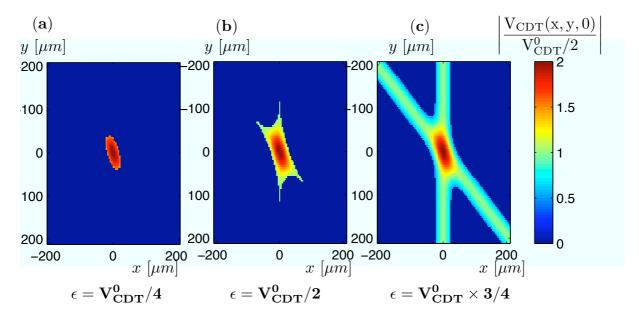
**Figure 2.** CDT potential in the z=0 plane, truncated at an energy  $\epsilon=V_{\rm CDT}^0/4$  (a),  $\epsilon=V_{\rm CDT}^0/2$  (b), and  $\epsilon=V_{\rm CDT}^0\times 3/4$  (c).
