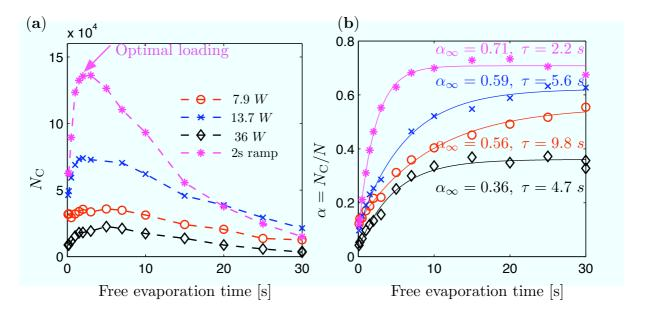
Figure 3. Evolution of the atom number in the center of the CDT (a) and the loading ratio  $\alpha = N_{\rm C}/N$  (b) in four different loading situations: low power (circles), highest power (diamonds),  $\sim 1/3$  of maximum power (crosses), ramping up in 2 s after loading at low power (stars). The loading ratio  $\alpha(t)$  is fitted with the function  $a(1 - e^{-t/\tau}) + b$ . The results of the fit  $\tau$  and  $\alpha_{\infty} = a + b$  are indicated in (b).
