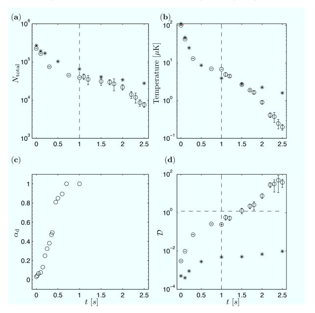
**Figure 5.** Evaporative cooling trajectories in the combined trap (CDT and dT) (circles) and in the CDT alone (stars). We show the time evolution of atom number N (a), temperature T (b), dimple filling  $\alpha_{\rm d}$  (c) and phase-space density  $\mathcal{D}$  (d).
