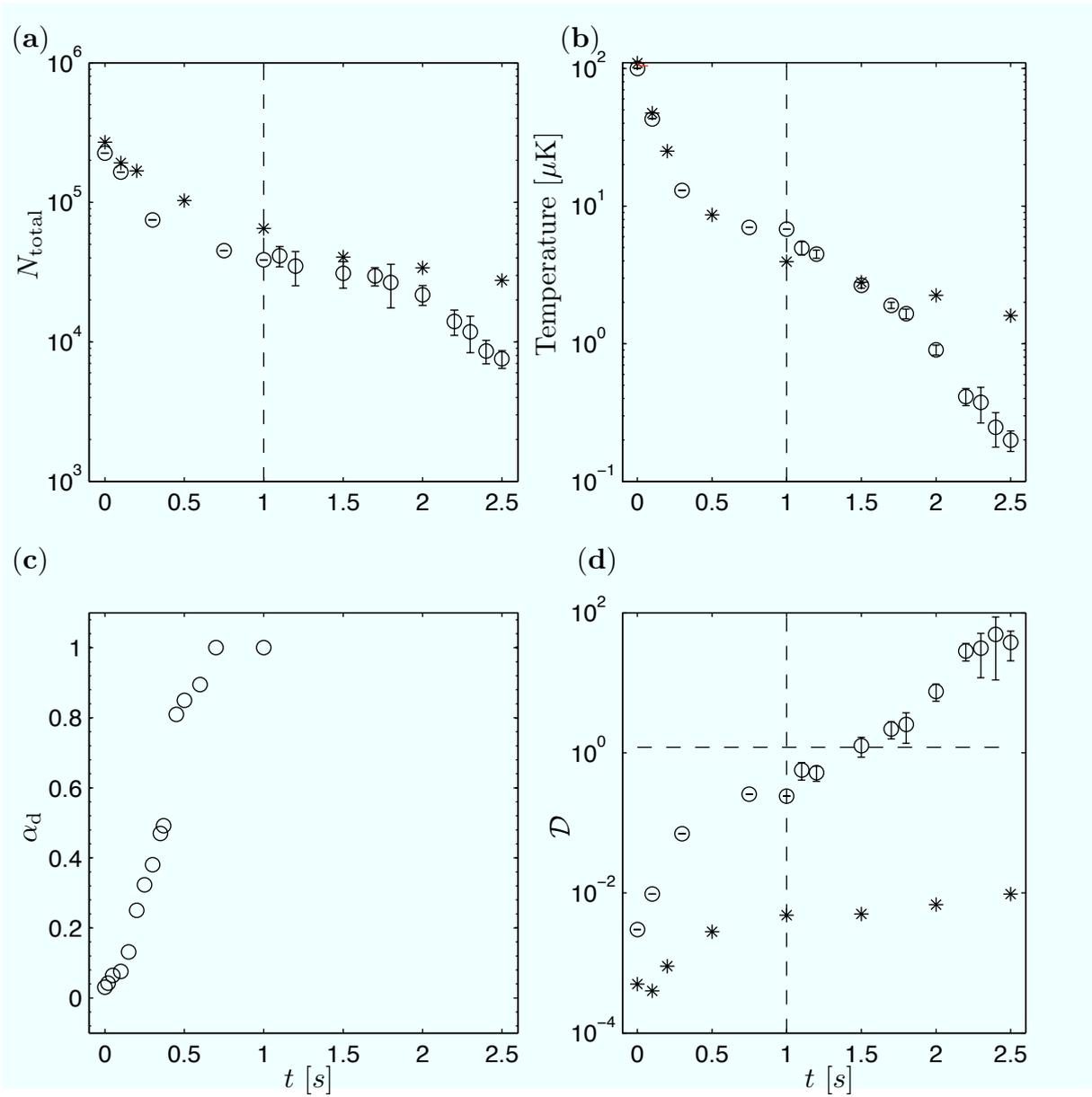
**Figure 5.** Evaporative cooling trajectories in the combined trap (CDT and dT) (circles) and in the CDT alone (stars). We show the time evolution of atom number  $N$  (a), temperature  $T$  (b), dimple filling  $\alpha_d$  (c) and phase-space density  $\mathcal{D}$  (d).
