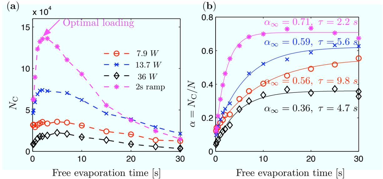
**Figure 3.** Evolution of the atom number in the center of the CDT (a) and the loading ratio  $\alpha = N_C/N$  (b) in four different loading situations: low power (circles), highest power (diamonds),  $\sim 1/3$  of maximum power (crosses), ramping up in 2 s after loading at low power (stars). The loading ratio  $\alpha(t)$  is fitted with the function  $a(1 - e^{-t/\tau}) + b$ . The results of the fit  $\tau$  and  $\alpha_\infty = a + b$  are indicated in (b).
