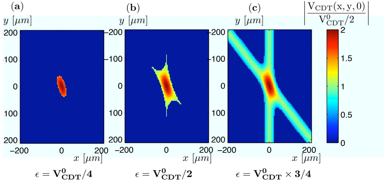
**Figure 2.** CDT potential in the  $z = 0$  plane, truncated at an energy  $\epsilon = V_{\text{CDT}}^0/4$  (a),  $\epsilon = V_{\text{CDT}}^0/2$  (b), and  $\epsilon = V_{\text{CDT}}^0 \times 3/4$  (c).
