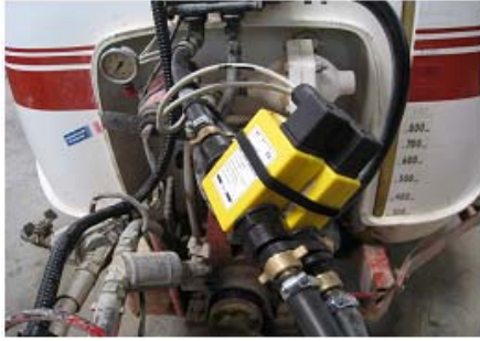
Figure 3: electro magnetic flow-rate meters © Cemagref 2009
