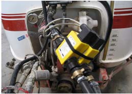
Figure 3: electro magnetic flow-rate meters © Cemagref 2009
