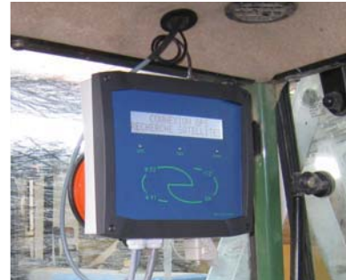
Figure 5: On board IHM system © Cemagref 2009
