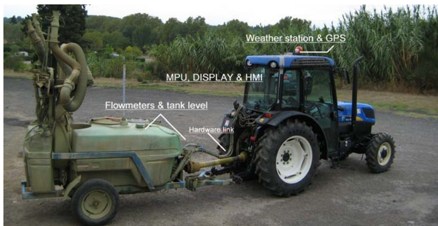
Figure 2: tractor – sprayer equipment, the tractor MPU © Cemagref 2009
