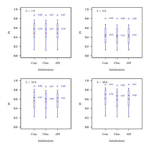
**Fig. 5.** Performance (persistence index) obtained by the model on 178 catchments, according to the initialization modes: continuous or event-based (climatic and API) strategies with a pre-forecast period lasting 360 h. Results are displayed for lead times ranging from 1 to 48 h.
