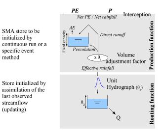
**Fig. 2.** Structure of the GRP model. The SMA store has to be initialized while the routing store level is updated when used in forecasting mode. *PE* and *AE* are potential and actual evapotranspiration.  $\theta_i$  are model parameters: a volume adjustment factor, the capacity of the routing store and the base time of the unit hydrograph.
