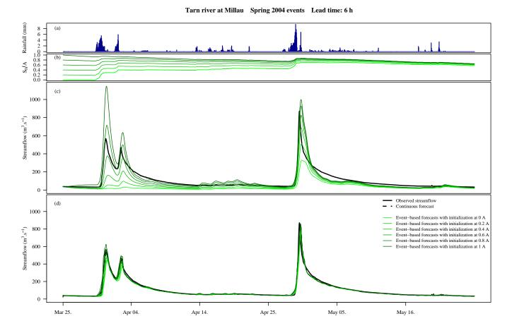
**Fig. 6.** (a) Precipitation during spring 2004 events. (b) Changes in the production store level after its initialization at different values on the 25 March 2004: there is convergence mainly during showers. Different initializations lead to very different forecasts when no updating technique is applied (c), whereas forecasts depend much less on the initial production store content when the model is updated (d).
