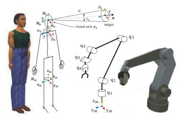
Figure 10. Manikin skeleton and robot kinematics; visibility cone and target definition.
