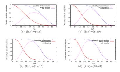
Fig. 3. Probability to rebuild a block as a function of the PLR for various FEC codes
