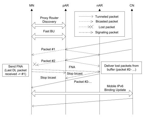
Fig. 1. The SafetyNet protocol operation
