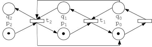
Figure 4: A 3-bit counter (without the reverse transitions).
