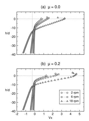
Figure 4. Velocity profiles for different values of  $\Omega$  (= 2 rpm, 6 rpm and 18 rpm) and two values of  $\mu_l$ : 0 (a) and 0.2 (b).
