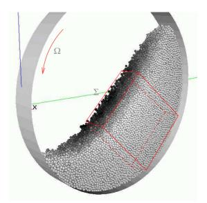
Figure 1. Typical snapshot of a 3D rotating drum. Its radius and its rotation speed are respectively D = 250 mm and  $\Omega = 18$  rpm. It is filled with 13000 spheres of density  $\rho^0 = 2.7$  g.cm<sup>-3</sup> and diameter uniformly distributed in the interval [3 mm; 3.6 mm].
