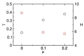
Figure 3. Velocity gradient (circles) and flowing thickness (squares) as function of  $\mu_l$  for  $\Omega = 6$  rpm.
