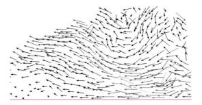
Fig. 9. Displacements in front of the sleeper.
