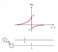
Fig. 2. Here we plotted the STDP additive synaptic weight updates as a function of the difference between the presynaptic spike time  $t_j$  and the postsynaptic spike time  $t_i$  plotted. The left part corresponds to Long Term Potentiation (LTP) and the right part to Long Term Depression (LTD).
