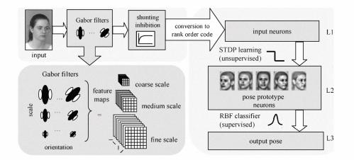
Fig. 4. Overview of the model used in [36]. The model consists of three major processing steps. Beginning with a preprocessing stage low level features are extracted and further converted into a rank-order code. Following, pose prototypes are learned from these temporal codes by applying STDP. After learning has converged, an RBF classifier is used to evaluate the responses from prototypical pose neurons (reproduced with permission from [36]).
