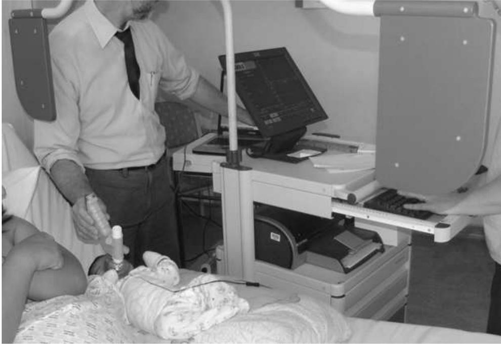
Figure 1a: Study setup, showing both FloRight vest and mask with ultrasonic flowmeter in place. The two fins of the magnetic field detector are shown suspended above the infant.
