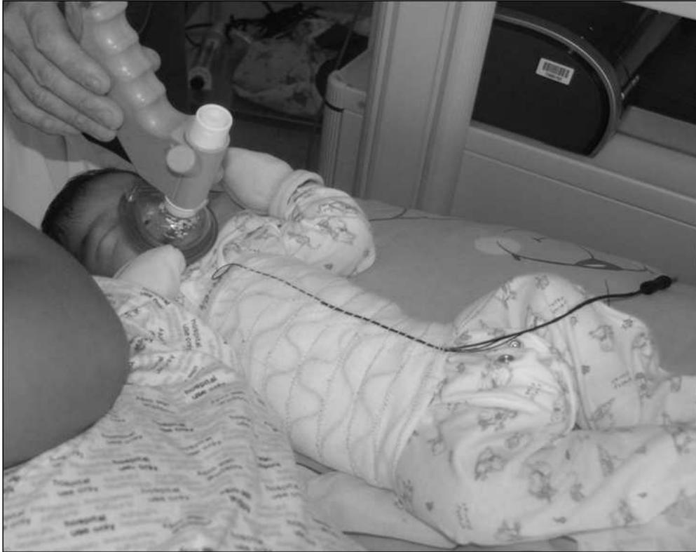
Figure 1: Study setup, showing both FloRight vest and mask with ultrasonic flowmeter in place.
