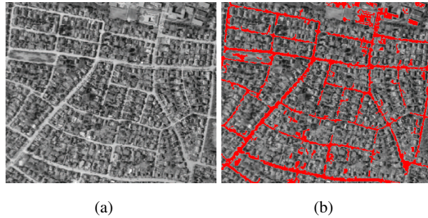
Figure 12: Second Test Results. (a) VHR IKONOS Example containing 300x300 pixels; (b) Road Map Result
