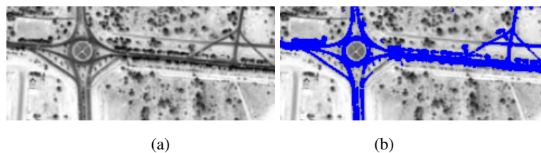
Figure 14: Third Test Results. (a) VHR IKONOS Second Example; (b) Road Map Result
