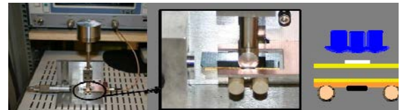
Figure 8. Photos and principle scheme of the mechanical bench for stress sensitivity characterization
