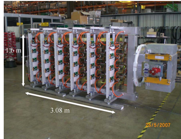
Fig. 11. View of the complete rectifier.
