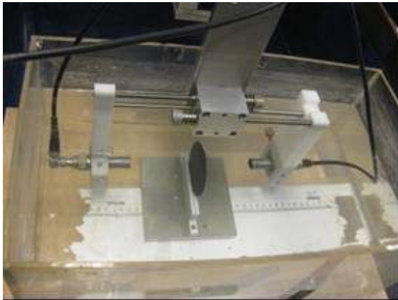
Figure 7. Ultrasonic characterization bench dedicated to non destructive control of the bonding interface
