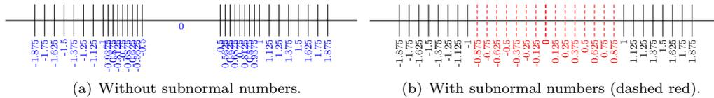
Fig. 3. The *tiny* floating-point format with and without subnormals (focus on 0).
