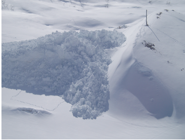
Figure 8.2: A wet-snow avalanche in front of the Ryggfonn catching dam that has piled up to a considerable height and also shows some tendency to divert sideways (photo: NGI).
