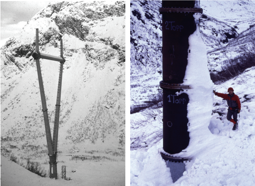
Figure 12.1: A mast built for studying impact forces on electrical power lines (left), and an instrument tower (right) that has just been hit by an avalanche in the Ryggfonn avalanche path in western Norway. The power line mast was broken several times by avalanches during the investigation period. (Photos: NGI.)
