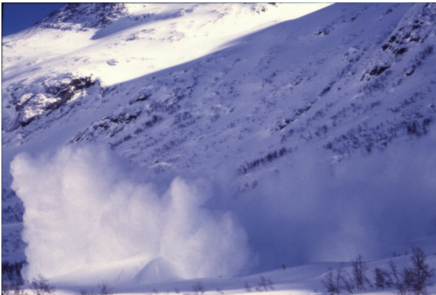
Figure 11.1: An avalanche impinging upon the catching dam at the NGI test site Ryggfonn. There is an obvious increase in depth as the avalanche hits the dam. (Photo: NGI.)
