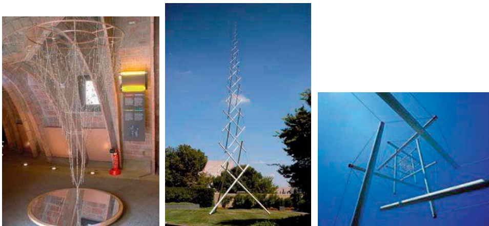
Figure 3. Catenary arch model (Gaudi museum) and the Needle Tower (tensegrity).
