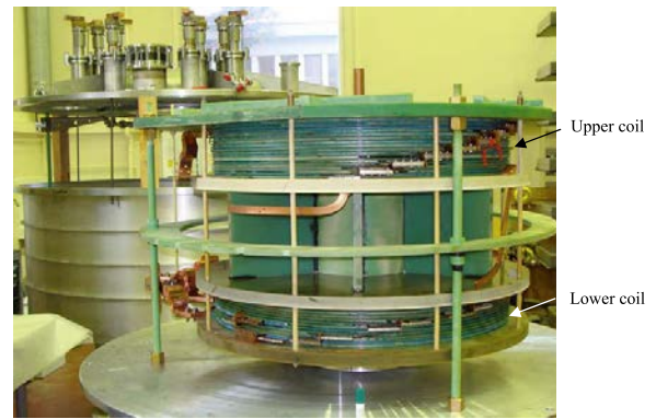
Figure 2. SMES II pancake arrangement forming two coupled coils.
