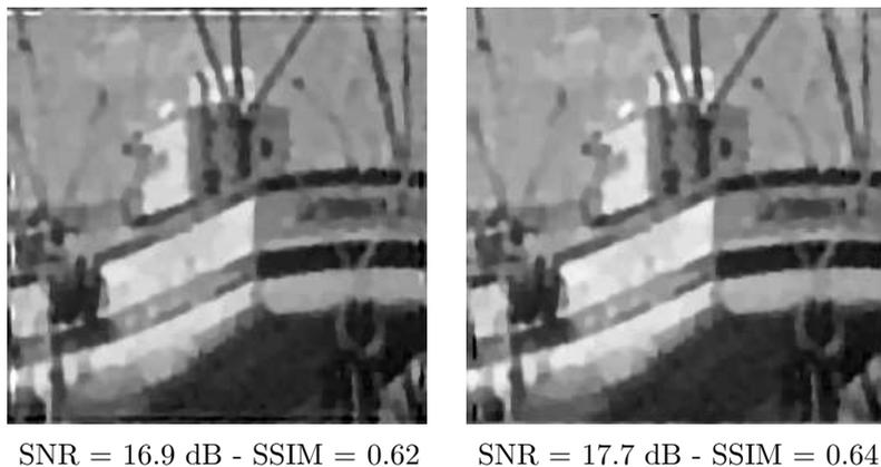
Figure 3: Periodic (left) and zero-padded (right) restoration.
