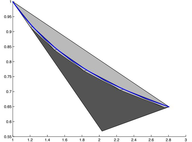
Fig. 4. Representation of exponential uncertainty and of construction of convex polytopes in the  $\phi_1(\delta\tau_k) - \phi_2(\delta\tau_k)$  plane, for  $\tau_{nom} = 0.1$ ,  $\delta\tau_k \in [0, 0.2]$ . The polytopic embedding in dark gray is obtained based on a 8th order Taylor approximation. In light gray we represent a polytopic embedding obtained based on a 8th order Taylor approximation applied on 5 subintervals.
