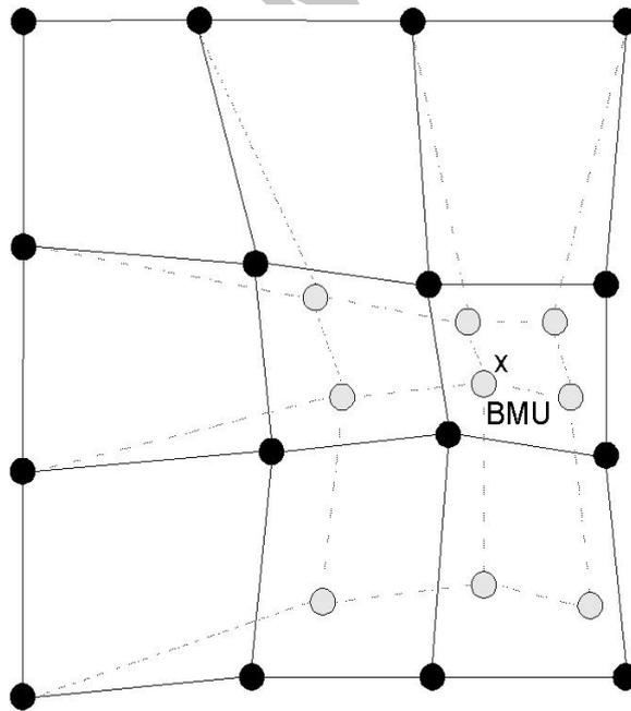
Figure 10: Updating the BMU and Its Neighbours towards an Input Pattern  $x$ . The Solid and Dashed Lines Correspond to the Neurons' Position Before and After Updating respectively.
