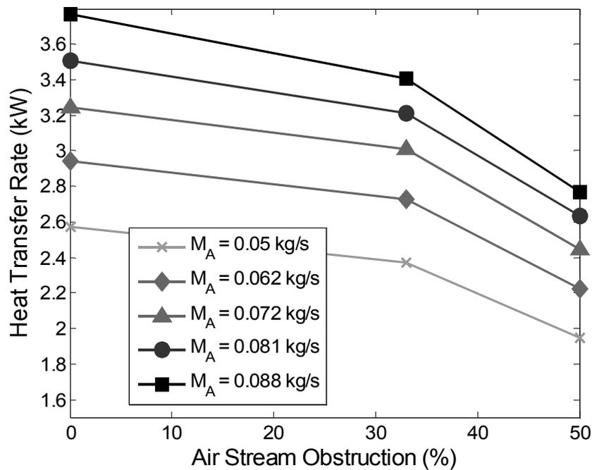
Figure 3: Effect of Inlet Obstructions on the Heat Exchanger Performance at Different Air Flow Rates
