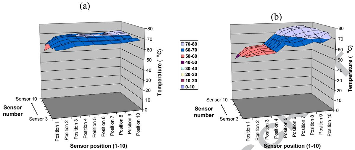
Figure 4: Air Temperature Distributions Over the Outlet Face of the Heat Exchanger
