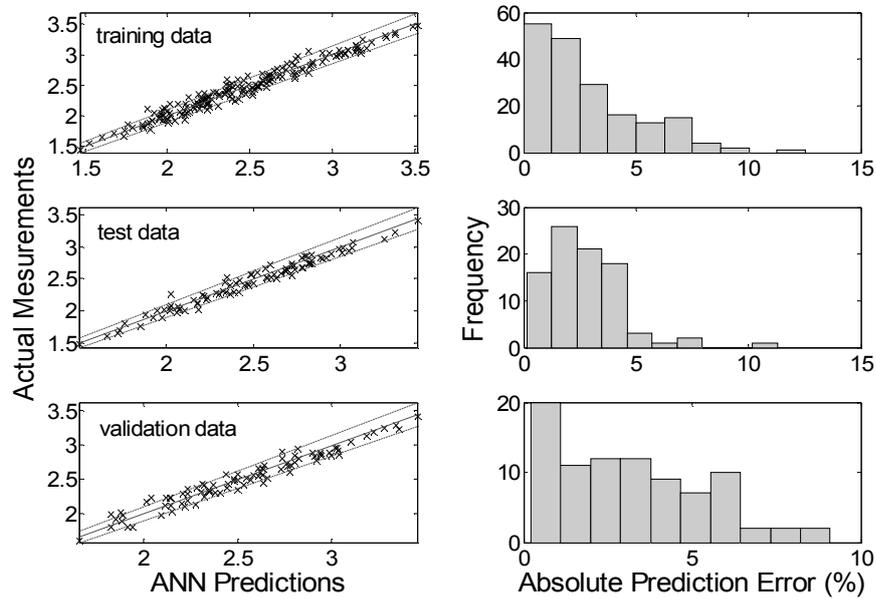
Figure 7: Representation of the Overall Heat Exchanger Performance by the NLR Model.
