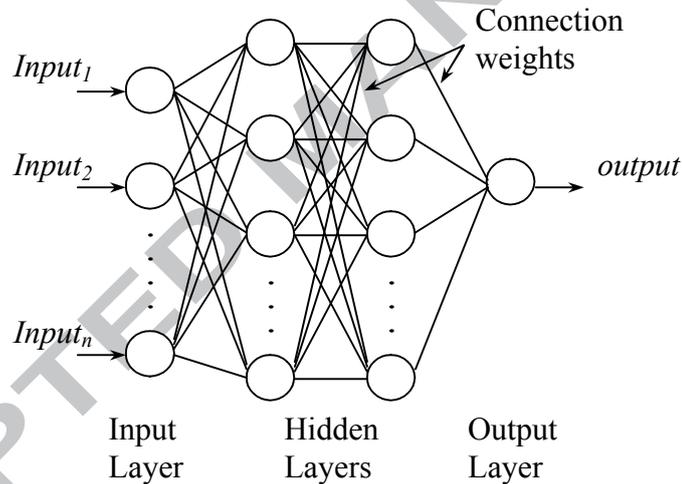
Figure 5: Schematic Representation of a Multi-Layer Perceptron ANN
