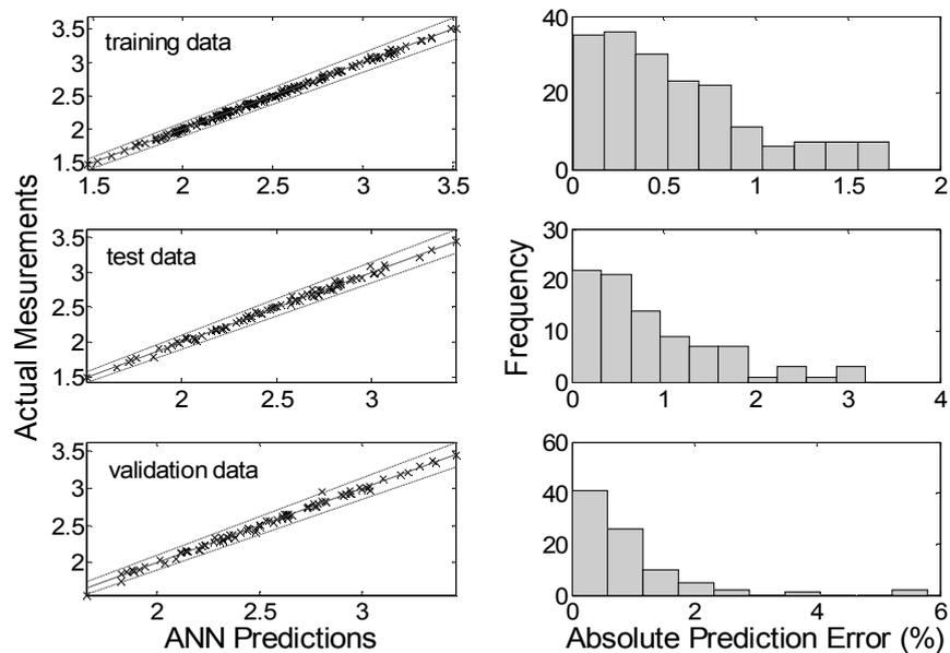
Figure 6: Representation of the Overall Heat Exchanger Performance by the ANN.
