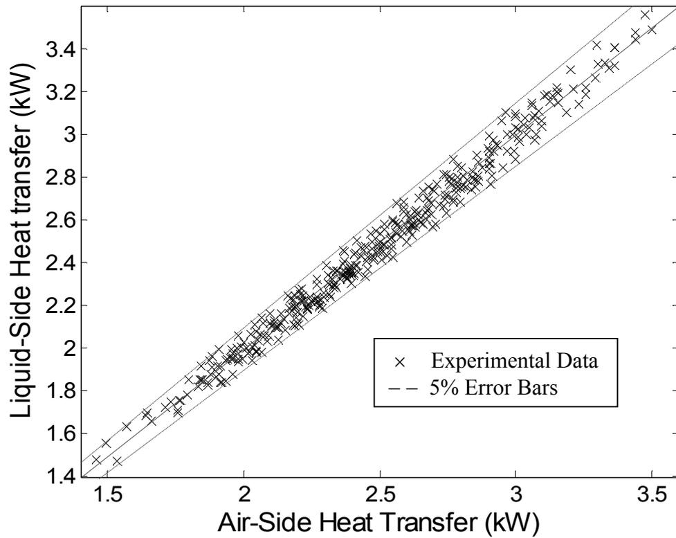
Figure 2: Comparison of the Liquid and Air-Side Heat Transfer Rates
