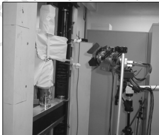
Fig. 12. Camera of the ARAMIS measuring system and lights
