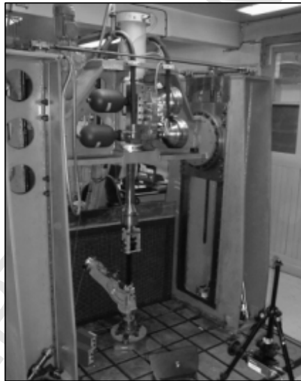
Fig. 9. Experimental fixture mounted on a high-speed hydraulic jack at ONERA-Lille
