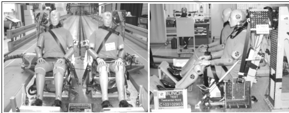
Fig. 3. Sled Test with two Hybrid III 95%ile dummies
