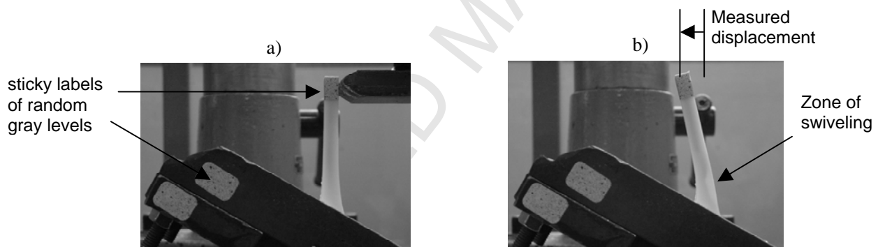
Figure 13: Digital images used by the DIC software to estimate displacements at the end of the structural component:
