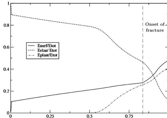
Fig. 17. Ratio of elastic energy  $E_{elas}$ , plastic energy  $E_{plast}$  and surface energy  $E_{surf}$  (dissipated + stored along the cohesive zones) to total energy  $E_{tot}$  (elastic + plastic + surface) vs ratio of time to final time for 30% hydrided Zircaloy-4.
