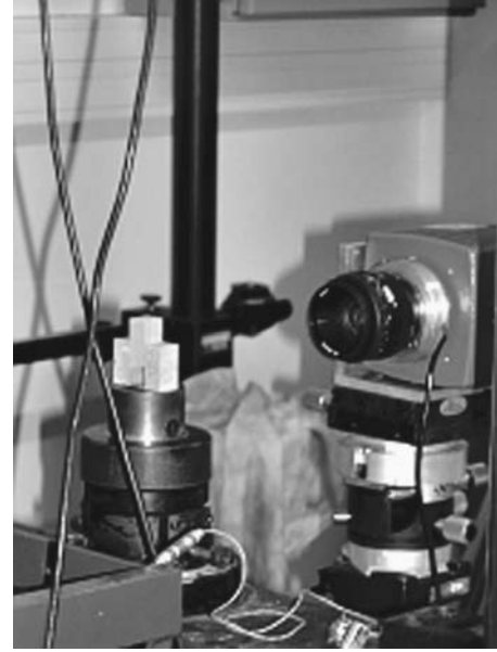
Fig. 3. Experimental device—testing machine coupled to a digital video camera
