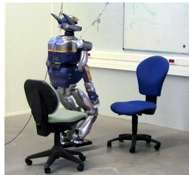
Figure 1: Humanoid Robot HRP-2 uses holonomic motion, or side-stepping, to pass between two chairs.
