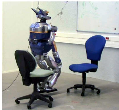
Figure 1: Humanoid Robot HRP-2 using holonomic motion (side-stepping) to pass between two chairs.
