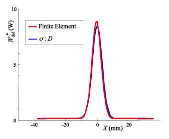
**Figure 8.** Longitudinal profiles of the deformation energy rate received by equally-spaced, 0.827 mm width, slices of the sample derived from kinematical data with the equilibrium equations (computed as  $\sigma : D$ ) and directly computed within the FE code.
