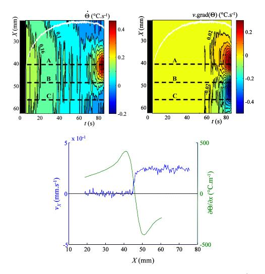
**Figure 5.** Time derivation of the temperature field: particular derivative  $(0.06 \,\mathrm{K \, s^{-1}})$  between two level curves (top left); convective term  $(0.04 \,\mathrm{K \, s^{-1}})$  between two level curves (top right); and Ox profiles of the longitudinal thermal gradient and velocity at  $t = 80 \,\mathrm{s}$  (bottom).
