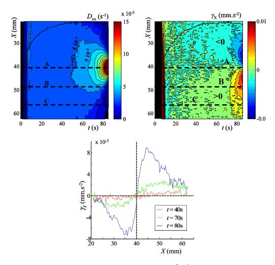
**Figure 9.** Spatiotemporal variation in  $D_{xx}(X, 0, t)$ ,  $10^{-3}$  s<sup>-1</sup> between two level curves (left) and  $\gamma_X(X, 0, t)$ , 0.002 mm s<sup>-2</sup> between two level curves (right). Different profiles of gx acceleration at t = 40, 70, 80 s are also shown (bottom).
