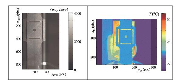
Figure 2. Calibration target: visible image (left); IR image (right).
