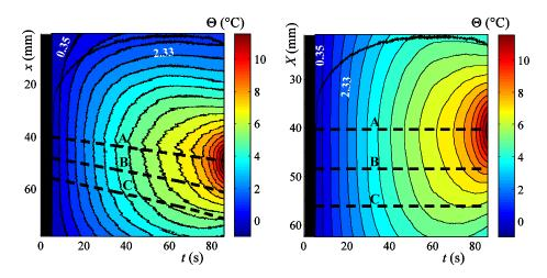
**Figure 4.** Temperature profile variations during a tensile test performed on a IF–Ti steel represented ( $\delta\theta$  between two consecutive level curves: 0.66 K). The deformed configuration (O, x, t) (left); and the reference configuration (O, x, t) (right).
