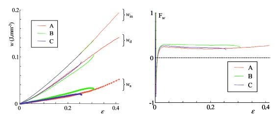
**Figure 13.** Energy balance at MSE A, B and C: variations in the stored  $w_s$ , dissipated  $w_d$  and inelastic  $w_{in}$  energies (left); local Taylor–Quinney ratio  $F_w$  (right).
