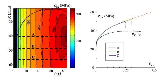
**Figure 10.** Mechanical response. Time duration of  $\sigma_{xx}(X, 0, t)$ , 25 MPa between two level curves (left); stress-strain diagrams of the three MSE A, B and C with the conventional stress-strain response of the specimen (right).
