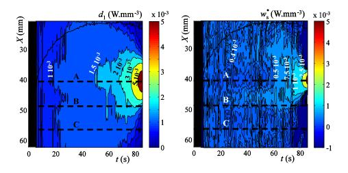
**Figure 12.** Spatiotemporal variations in  $d_1(X, 0, t)$  (left);  $w_s^{\bullet}(X, 0, t)$  (right).
