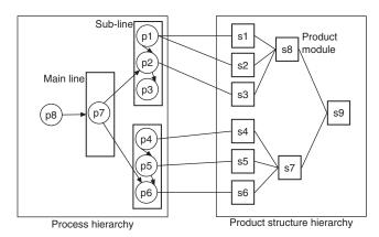
Figure 3. Modularization in production: multiple hierarchies.
