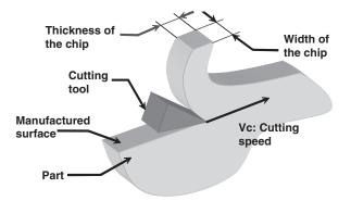
Figure 2. Representation of the material cutting process.
