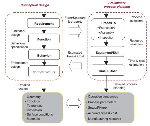
Figure 3. Design and process planning interfaces.
