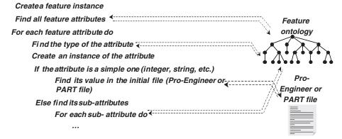
Figure 13. General algorithm for data exchange.
