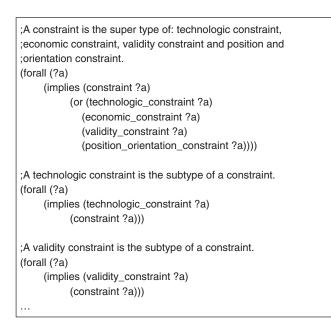
Figure 6. KIF statements for constraint classification.
