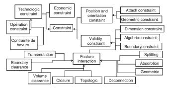
Figure 5. Constraint classification.
