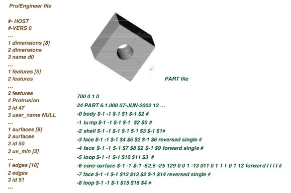
Figure 11. Data declaration in Pro-Engineer and PART files for a simple artifact.
