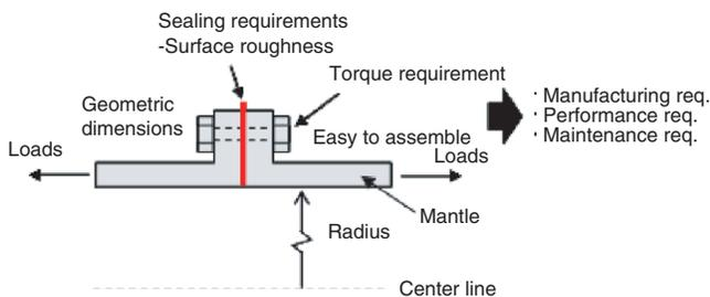
Figure 8. Two rotational symmetric jet engine component flanges.
