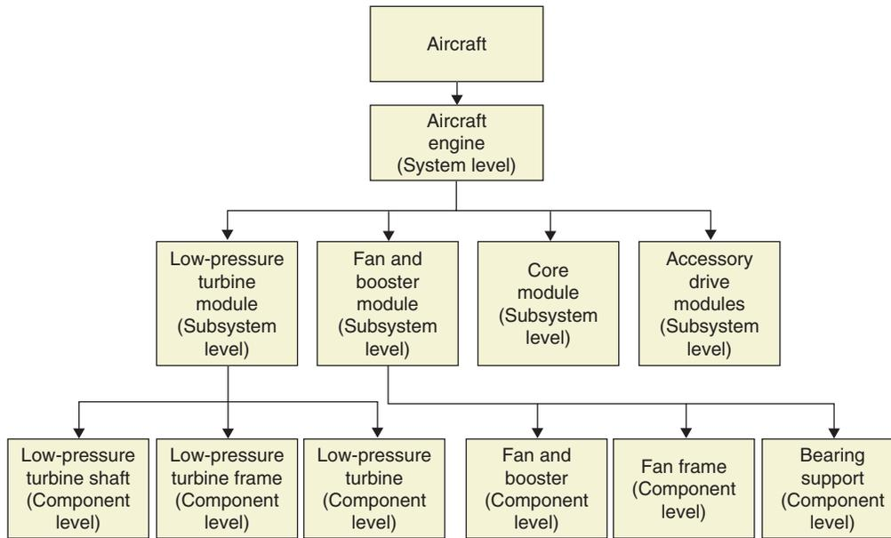
**Figure 1.** Excerpt from an aircraft system level overview.
