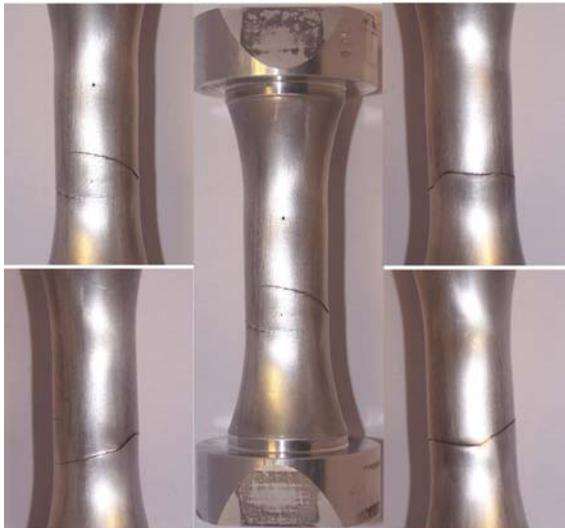
Figure 3. General view of a specimen at the end of its life showing various profiles.
