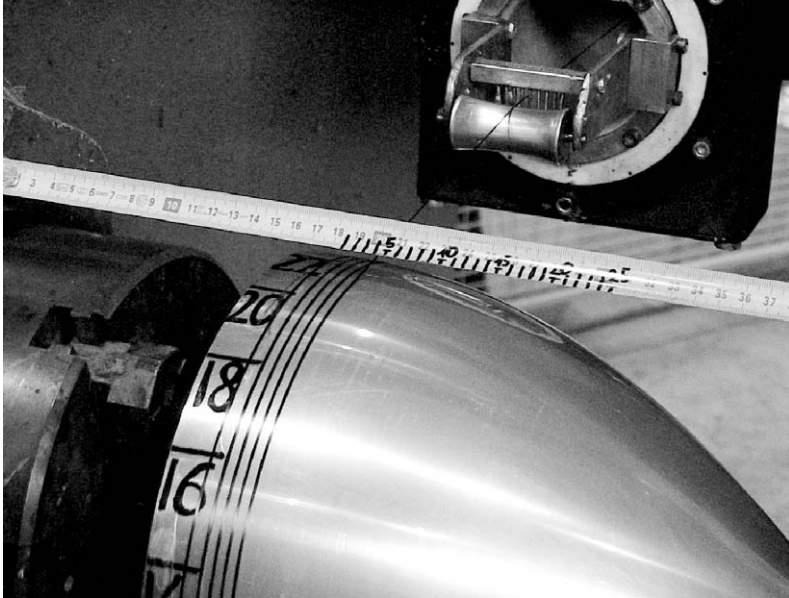
Figure 10. The mandrel with benchmarks for the carriage Z and the rotation C .
