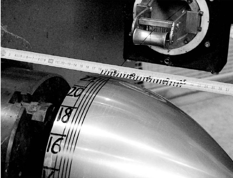
**Figure 10.** The mandrel with benchmarks for the carriage Z and the rotation C.
