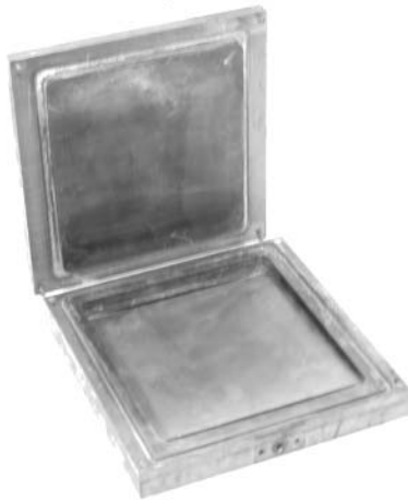
Figure 2. Experimental setup in laboratory scale, specially designed negative mold.
