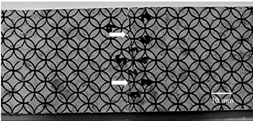
Figure 8. Shape fracture in a 50-mm wide blank.
