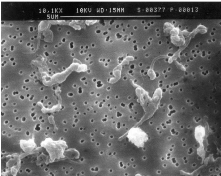
Figure 4. SEM image of submicron-sized polyethylene particles isolated from tissues of a patient of Group 1.
